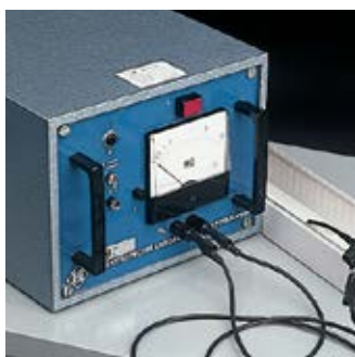
Apparatus for insulation resistance above 100 MΩ.
