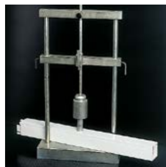
Apparatus for shock testing at low temperature.
