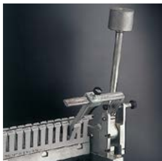
Apparatus for finger-removal and side-segment removal test.
