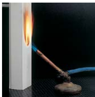
Apparatus for flame propagation resistance test.
