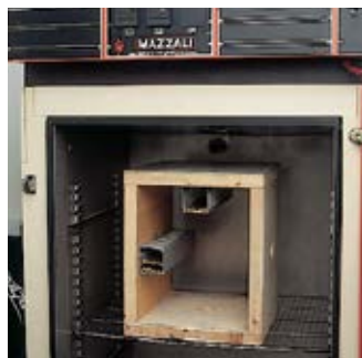
Cabin for age acceleration test.
