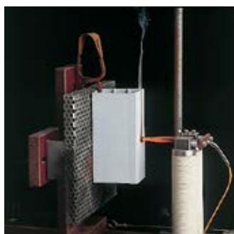
Apparatus for testing heat resistance (850° C) GWT.
